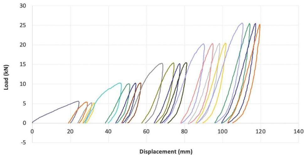
Figure 7. Four layers of geogrid – displacement vs load (Flaherty, 2020).
