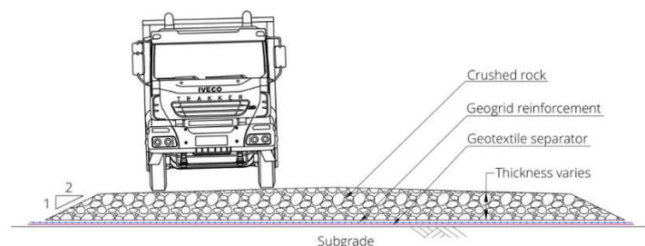
*Figure 1. Typical unpaved road cross section.*
